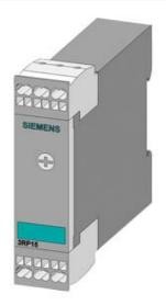
MULTIFUNCTION TIME RELAY IN CAGE-CLAMP TECH. 1 NO CONTACT DELAYED, 1 NO CONTACT NON-DELAYED, 3S...60S, AC/DC 24V, AC 100...127V
