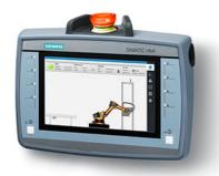
SIMATIC HMI KTP700F Mobile, 7.0" TFT display, 800x 480 pixel, 16m colors, key and touch operation, 8 function keys, 1x PROFINET/Industrial Ethernet interface, 1x multimedia card, 1x USB, Key-operated switch, acknowledgement button, 1 emergency stop/stop button configurable from WinCC Comfort V13 SP1
