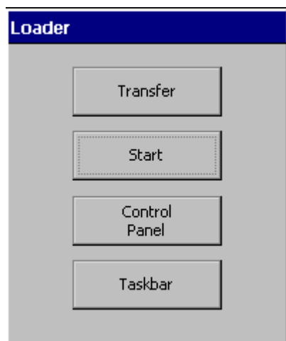
Figure 6-1 HMI device loader
