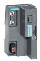
SIMATIC DP, IM151-7 CPU for ET200S, 128 KB work memory with integrated PROFIBUS DP interface (9-pole D-sub socket) as DP slave, without battery SIMATIC MMC required
