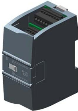
SIMATIC S7-1200, Digitale E/A SM 1223, 8 DI/8 DO, 8 DI DC 24V, Sink/Source, 8 DO, Relais 2A
