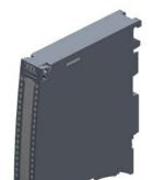
SIMATIC S7-1500 Analog input module AI 4xU/I/RTD/TC ST, 16 bit resolution, Accuracy 0.3%, 4 channels in groups of 4; 2 channels for RTD measurement; Common mode voltage 10 V; Diagnostics; Hardware interrupts; Delivery including push-in front connector, infeed element, shield bracket, and shield terminal
