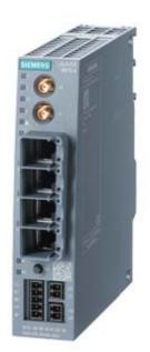
SCALANCE M876-4 4G router; for the wireless IP communication from Ethernet-based Programmable controllers via LTE (4G) mobile radio optimized for use in Europe, VPN, Firewall, NAT; 4-port switch; 2x SMA antennas, MIMO Technology; 1x digital input, 1x digital output; observe national approvals!
