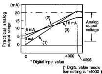
(2) Relation between the offset/gain values and the analog output
