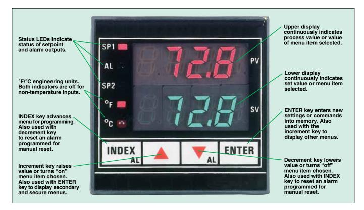
The CN76000 ½ DIN controllers provide economical control for a wide variety of processes, including heating, cooling, and heat/cool. When used with the proper transmitters, these devices can also control pressure, flow, humidity, motion, or pH. The front panel is NEMA 2, 3R, and 12 rated for waterproof protection and is corrosion resistant.
