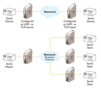
Each unit passes data from its serial interface to the serial interface of the other unit. This enables long distance serial communication using preexisting networks.
