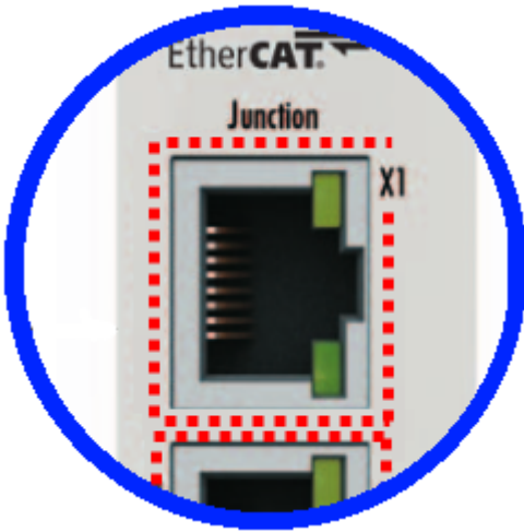
Abb. 6: Fast-Hot-Connect Ports des EK1122-0080
