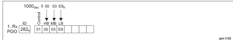
Fig. 12.5-18 Example - How to assign a comparison value to channel 0 when using SSI interface
