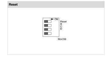
The reset switch should be set to 'ON' for approx.  $\frac{1}{2}$  s, causing the station to load the USER-data from the EPROM and to start operation under defined starting conditions.
