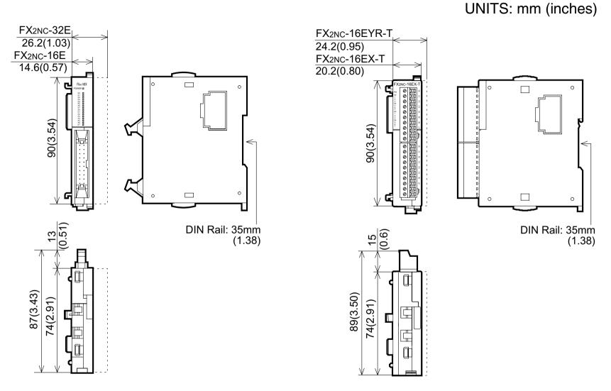
FX<sub>0N</sub>, FX<sub>2N</sub> Extension block dimensions  $\rightarrow$  (See sec. 3.7)
