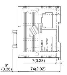
FX2NC-232ADP FX2NC-485ADP \* : FX2NC-485ADP is 4(0.16)
