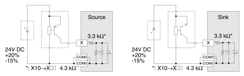
Figure 5.3: FX2NC Main unit and FX2NC Extension block
