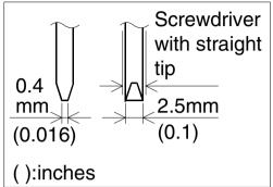
Use a small commercial screwdriver of the size shown on the left. Make sure that the tip is straight, and is not broadened.
