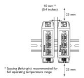
This unit uses convection cooling. To avoid obstructing the airflow around the unit, use the following spacing rules. Minimum spacing 25 mm (1.0 inch) above / below and 10 mm (0.4 inches) left /right the unit. Spacing is recommended for the use of unit in full operating temperature range and service life.
