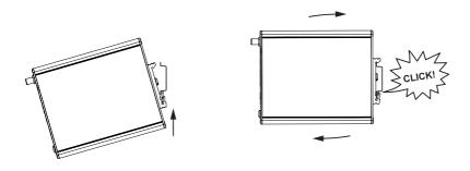
The MRD-315 and MRD-415 includes integrated mounting flanges and can be attached to a panel or tray by means of screws, using the slots provided. Alternatively the MRD-315 and MRD-415 can be DIN rail mounted, using the DIN rail mounting kit.
