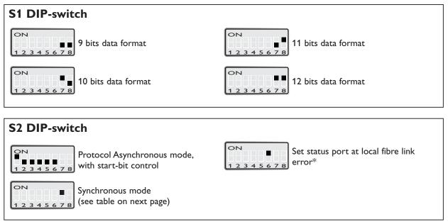
\* SW 2:6 ON: The status relay only change status in the unit that is connected to the receive side.
