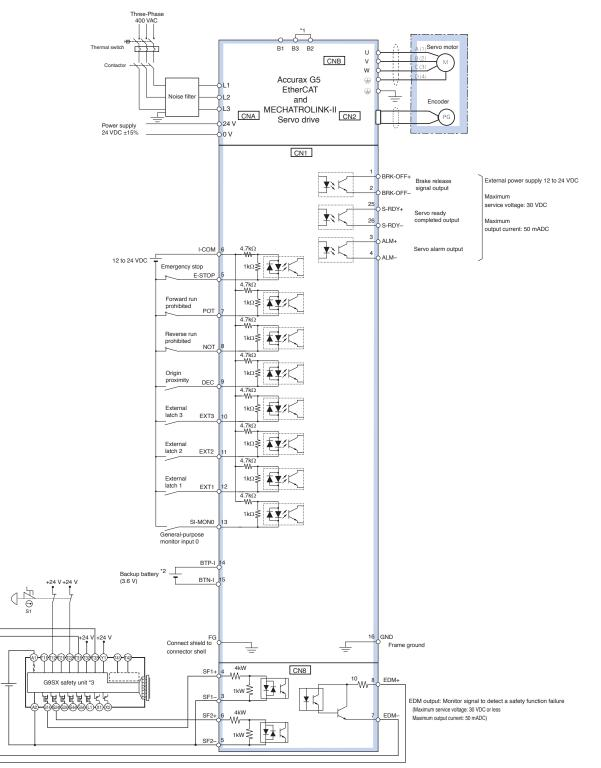
\*1 Normally B2 and B3 are short-circuited. If the internal regenerative resistor is insufficient, remove the wire between B2 and B3 and connect an external regenerative resistor between B1 and B2.
