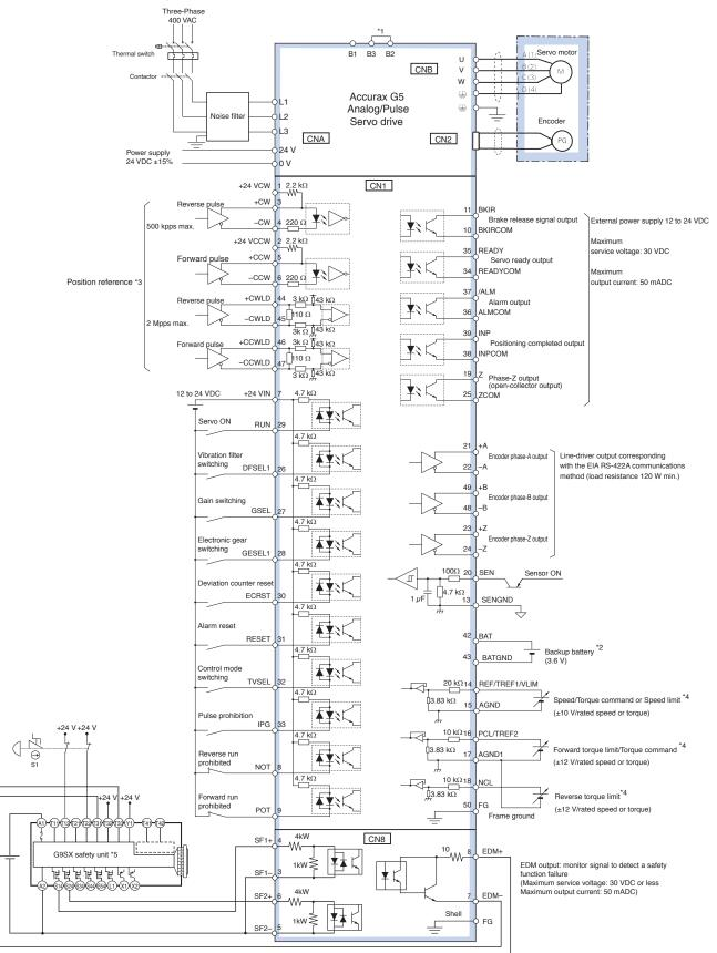
\*1 Normally B2 and B3 are short-circuited. If the internal regenerative resistor is insufficient, remove the wire between B2 and B3 and connect an external regenerative resistor between B1 and B2.
