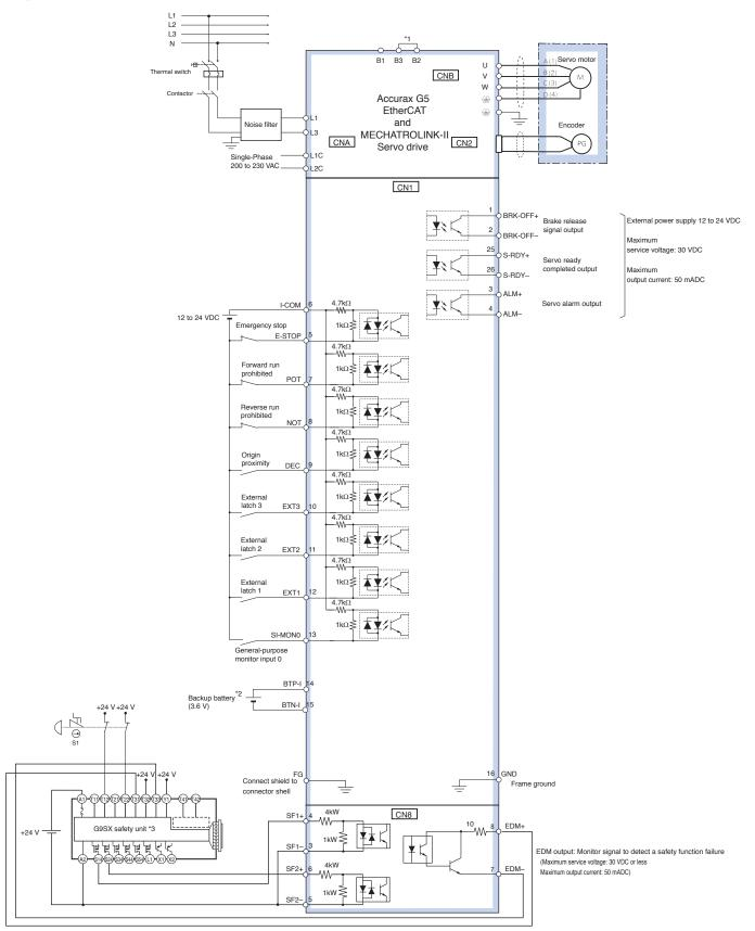
\*1 For serve drives from 750 W, B2 and B3 are short-circuited. If the internal regenerative resistor is insufficient, remove the wire between B2 and B3 and connect an external regenerative resistor between B1 and B2.
