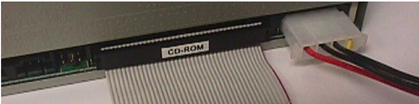
Figure C.7: Plug Power Line into CD-ROM Drive
