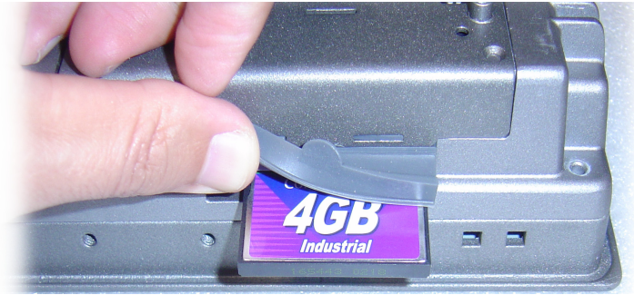
Figure 2.1: Install CompactFlash memory card
