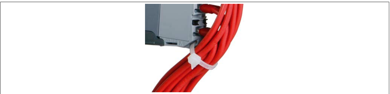
Figure 16: Slots through which the cable ties are fed
