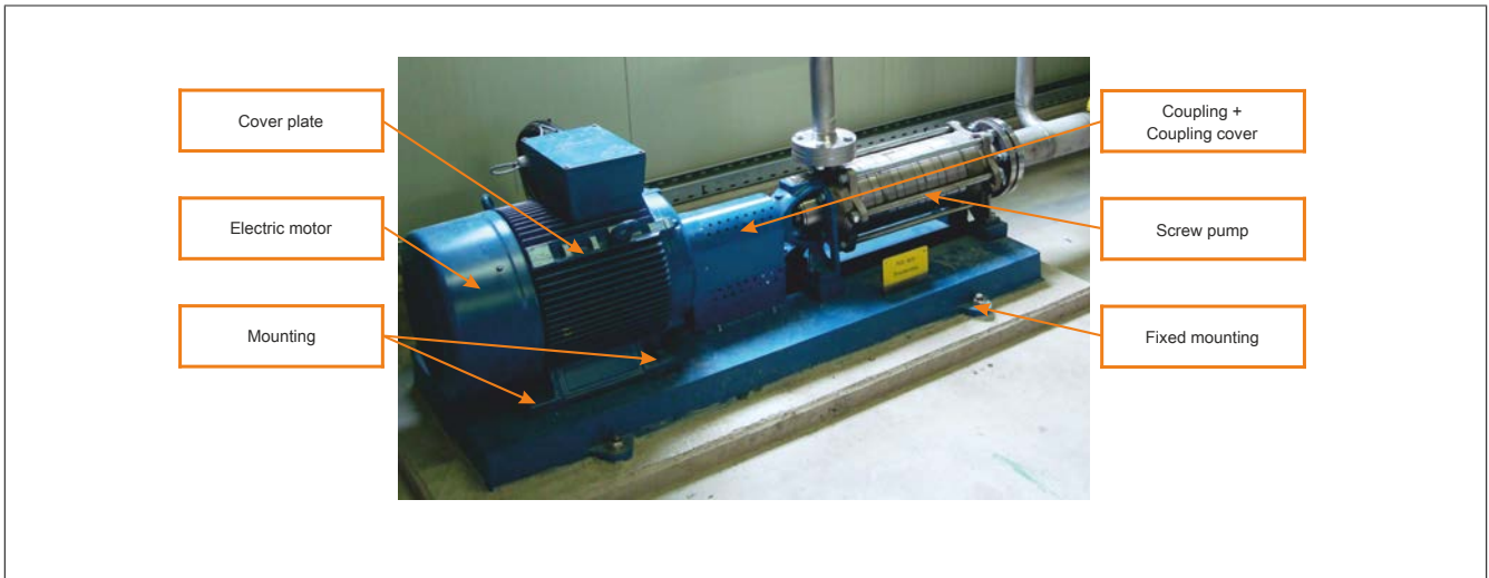
Figure 262: Structure of a pump drive
