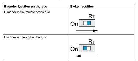
**NOTE:** If the line terminator is set to "ON", the "BUS OUT" terminals *Wiring the Bus and the Power Supply, page 19* shall be disconnected.
