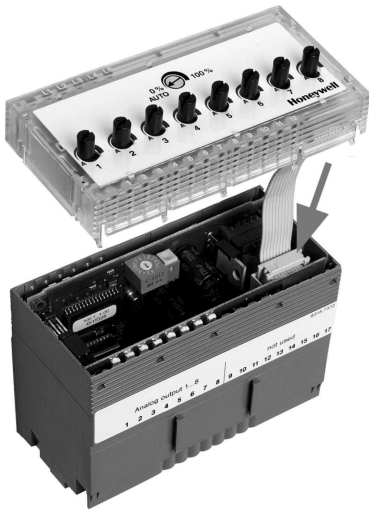
Fig. 20. Manual override connector socket location
