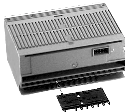
Fig. 14. Inserting coding comb into I/O module
